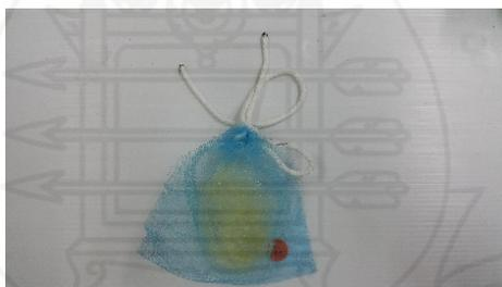
**Figure 2.** Plastic bag containing amidoxime fibers
